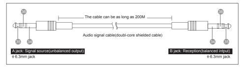
(3) Connection for Unbalanced to Balanced XLR transmission cable: Practical example: the recording output of IT-12M4 "REC. OUT" (unbalanced output) to PA system or media recording input XLR interface (balanced input).
